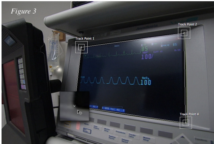
Figure 3: Place the center of each track point around a feature with clearly defined shapes, sharp edges, and good contrast, such as the corners of the computer screen's bezel.
