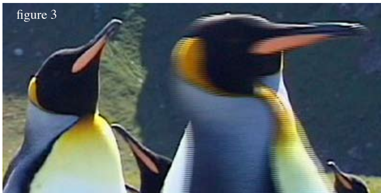
Figure 3: The "comb teeth" pattern around the moving penguin on the right tells us this clip is interlaced. Note that since the penguin on the left is not moving, we don't see the comb teeth pattern; you need motion to actually determine if a clip is progressive or interlaced. Clip VPE111 from the Artbeats Penguins V-Line collection.
